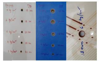
Fig 8: Ceramic tiles drilled at different Pressure, SOD, and AFR
